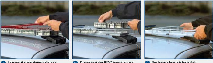
Remove the top dome with only four screws.
