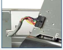
Minimal Board-to-Board **Connections** reduce about 85% of potential failure points. ROC uses a printed circuit board in one assembly to significantly reduce the electrical connections found in a typical lightbar.
